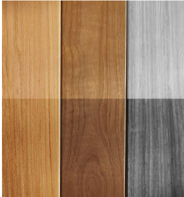
Fresh, darkened, grayed. Top not oiled, bottom oiled.
